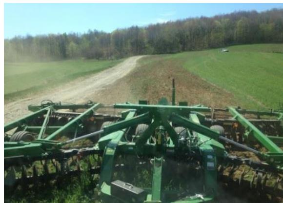
**Figure 3. Vertical tillage.**
