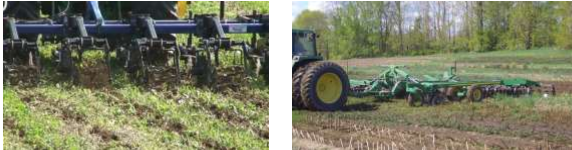
Figure 1. Blu-Jet Coulter Pro strip tillage, left, and John Deere 2623 VT vertical tillage, right.
