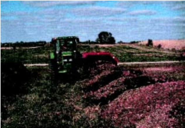
Figure 6b. Using a tractor-pulled windrow turner to mix cannery wastes with sawdust and municipal leaves
