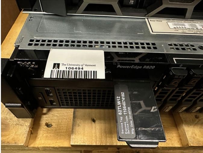
Picture # 5- **Recommended**- server tag is folded correctly and is forward facing on the asset, allowing the adhesive to go on the metal and the tag to flop up and down.
