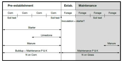
**Figure 1. Example of the time of soil testing in a corn/hay crop rotation.** (Source: Penn State University Extension)
