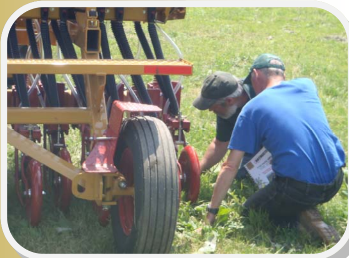
Jeff Carter helping a farmer calibrate the no-till drill.
