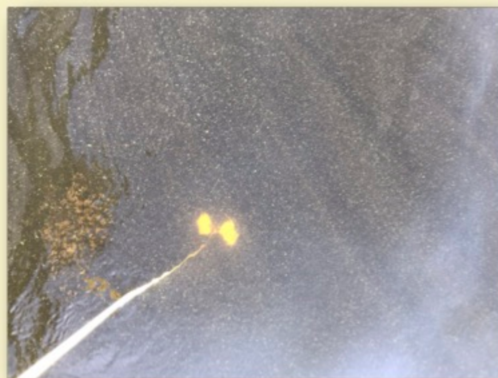
A secchi disk is used to monitor water clarity
