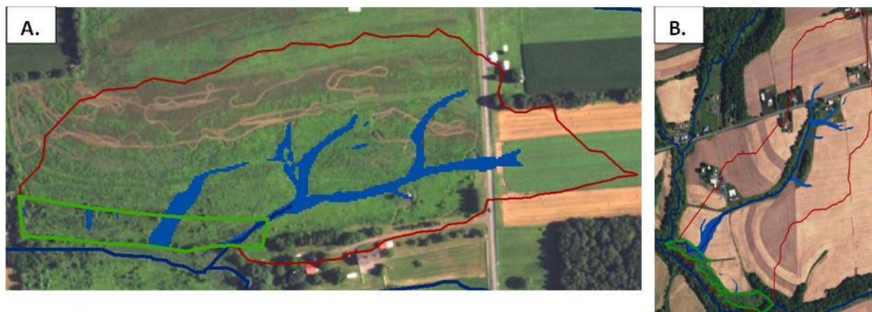
Figure 19. Flow Accumulation for CP22 contributing drainage areas in the Mahantango Creek watershed: (A. two concentrated flowpaths that fully transect the buffer, with the largest flowpath draining approximately 59% of the contributing area, and (B. one major concentrated flowpath where grassed waterway is implemented along with CP22 to maximize efficiency.
