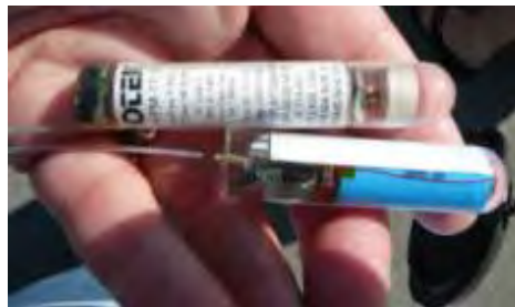
Figure 2 - Lotek transmitters (Dual acoustic, above , Radio, below ).
