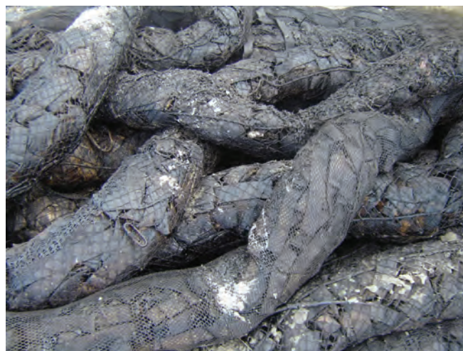
▲ Figure 3: Strips of polypropylene enclosed in netting. The loose inhomogeneous structure of the boom may allow oil to readily penetrate into the structure allowing inner surfaces to adsorb oil but the enclosing netting may be easily damaged.
