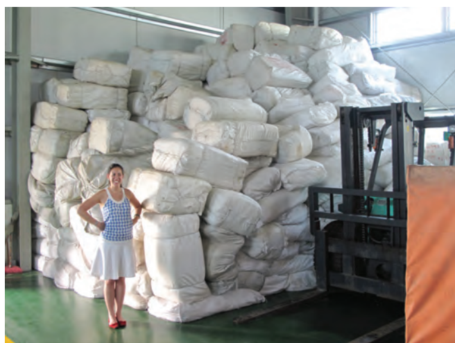
▲ Figure 8. Sorbent materials by their nature are bulky products. Storage and transport before, during and after a response to a spill can pose logistical and cost issues.
