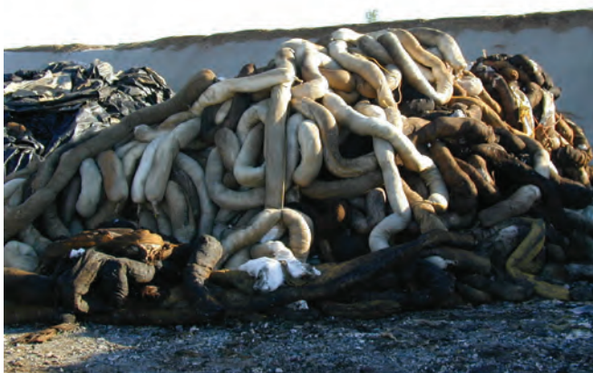
▲ Figure 15: Used sorbent piled in a temporary storage site. Compression will cause recovered oil to be squeezed from the boom and care is needed to avoid secondary contamination.
