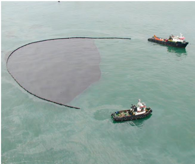
▲ *Figure 8: Inflatable boom deployed in a U configuration between two vessels to contain a heavy crude oil. Recovery of the oil will bring the operation to a successful conclusion.*
