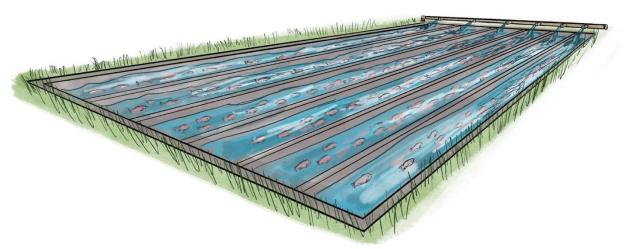
Figure 3. Example drawing of a flow-through raceway system.
