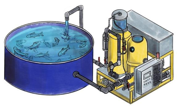
Figure 2. Example drawing of recirculating aquaculture system (RAS)<sup>2</sup>
