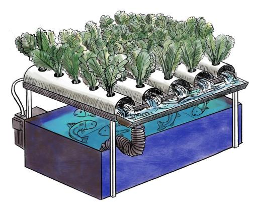
Figure 5. Example drawing of an aquaponics system.
