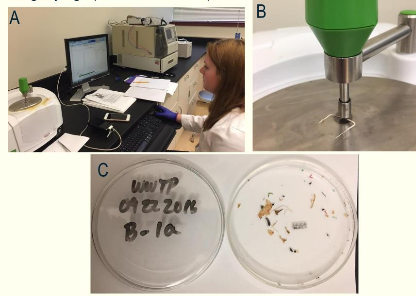
Figs. 1. A) Perkin Elmer FT-IR machine connected to a PC, B) FT-IR of a white fiber, C) dried sample from wastewater treatment plant about to undergo FT-IR.
