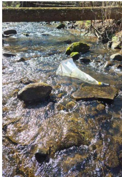
Surber sampler placed in a high-flow riffle area
