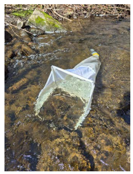
Surber sampler placement in stream flow
