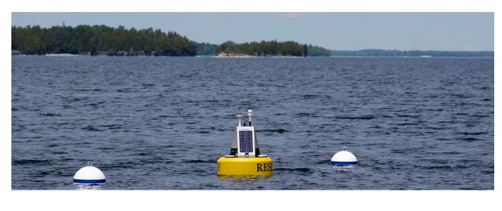
A data buoy (image, above right) was deployed during the 2016 field season near Valcour Island, just north of the Main Lake 'Site 19' discussed in **Section 1**. The data buoy measured surface air temperature, wind speed and direction, and air pressure, while also observing water temperatures between the surface and 50 m depth with 1 m resolution.
