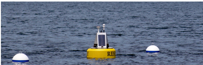
Water temperature and meteorological research buoy (Photo, E. Leibensperger)
