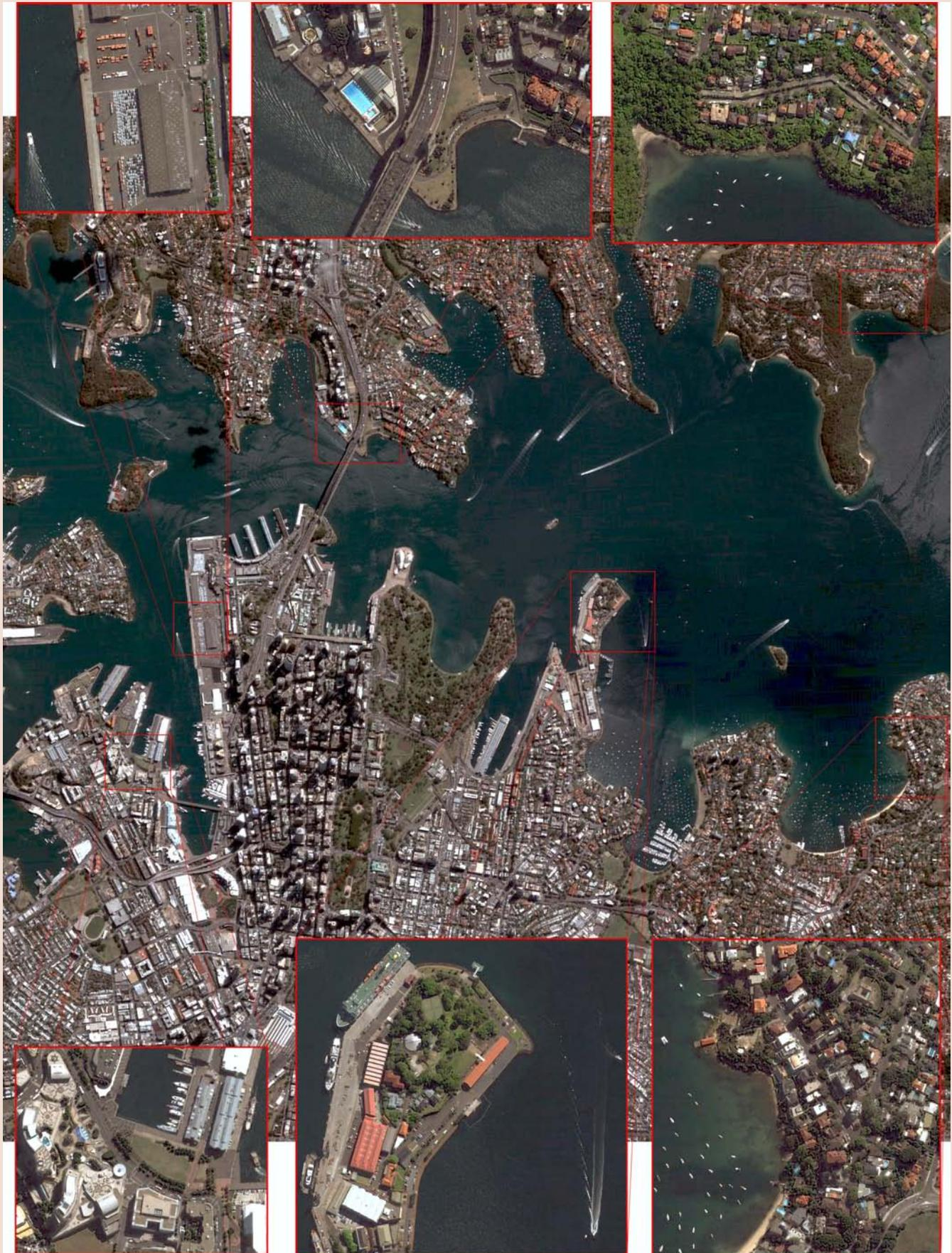
Figure 4. Original QuickBird 2.4m MS natural color image of Sydney, Australia, with subsets of fused 0.6m color image of the statistics-based fusion (top middle; bottom left and right) and subsets of 0.6m color enhanced fusion image (top left and right; bottom middle).
