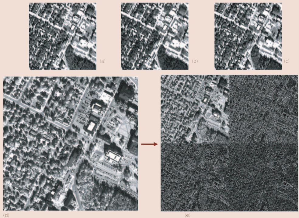
Figure 3. Original IKONOS MS band 1 (a), band 2 (b), band 3 (c), Pan (d), and the wavelet decomposition of the original Pan (e) with a low-resolution Pan (upper left) and wavelet coefficients (spatial details) in horizontal, vertical and diagonal directions (upper right, lower left, and lower right).
