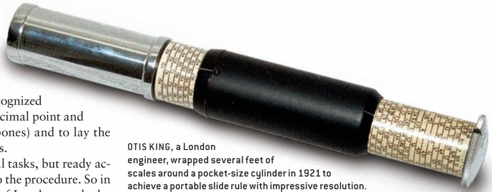
OTIS KING, a London engineer, wrapped several feet of scales around a pocket-size cylinder in 1921 to achieve a portable slide rule with impressive resolution.
