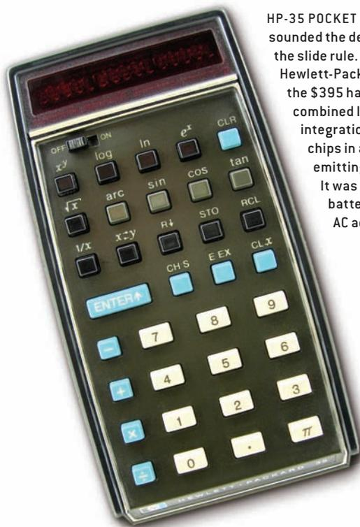
HP-35 POCKET CALCULATOR sounded the death knell for the slide rule. Introduced by Hewlett-Packard in 1972, the \$395 handheld device combined large-scale integration circuits (six chips in all) with a light-emitting diode display. It was powered by batteries or an AC adapter.
