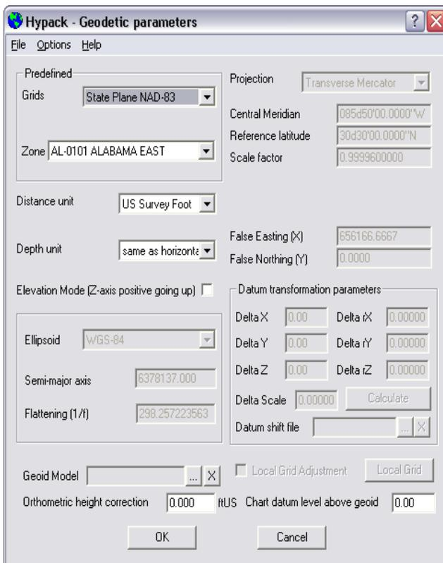
The first thing many users notice is that our definition of NAD-83 uses WGS84 as ellipsoid while the standard definition uses GRS-80 ellipsoid. Here are, for reference, the defining parameters for the two ellipsoids:
