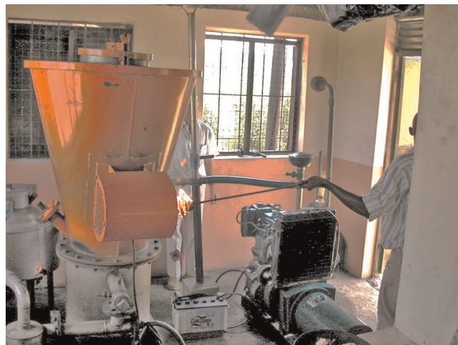
Figure 8. 10 kW dual-fuel mode gasifier for electricity production
