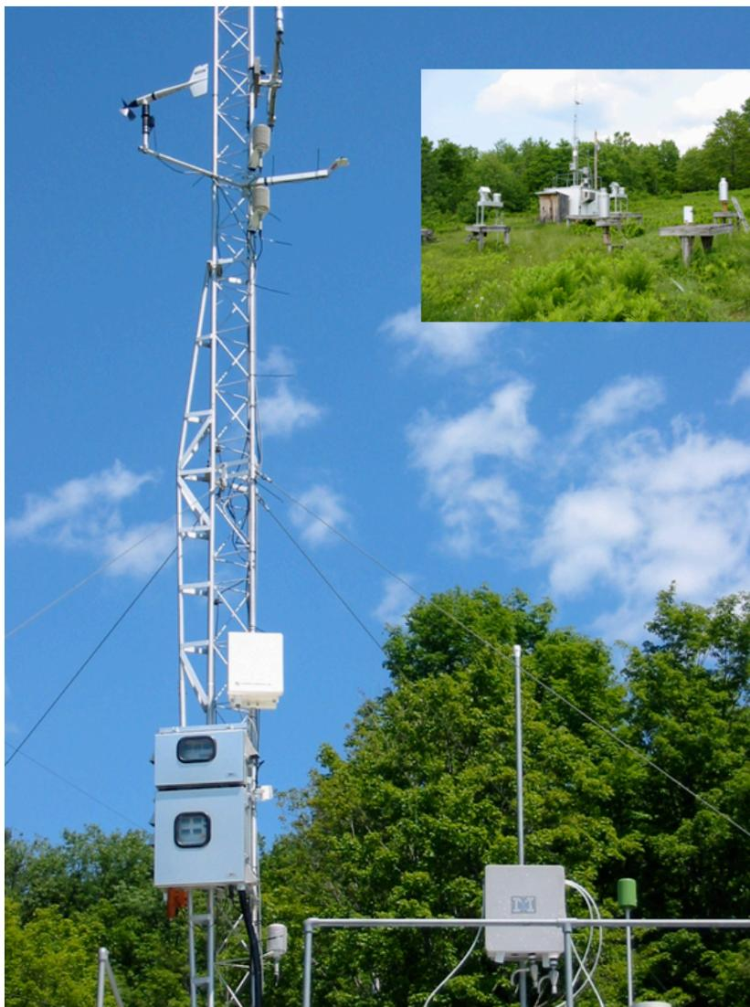
**Figure 2.** Sampling heads for RGM, GEM, and particulate mercury were located on the met tower fixed to the instrument shelter (see inset) at the Underhill, VT Air Quality Site in April of 2005.
