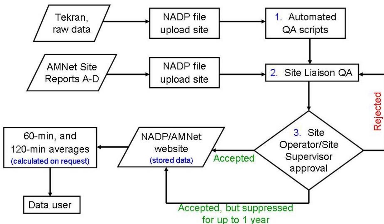
**Figure 2.** AMNet Quality Assurance and Data Flow Process.
