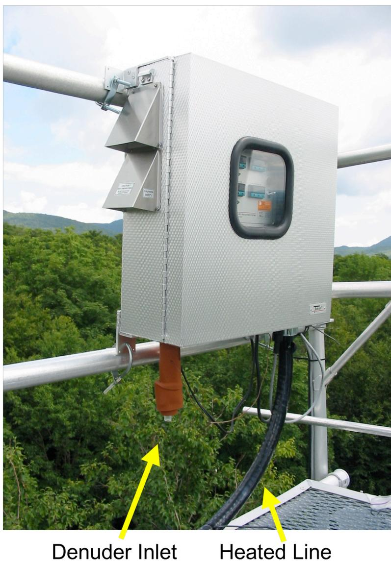
**Figure 1.** Initial deployment of RGM sampling head on the forest canopy observation tower in 2004.
