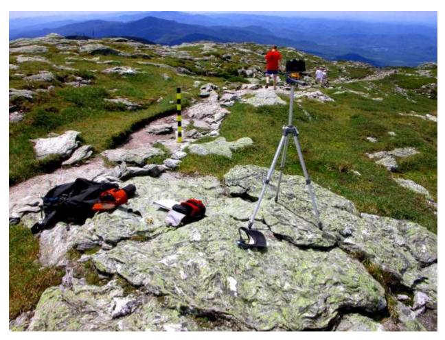
Standard phototransect setup: Camera and tripod on right, meter board 5 meters away on left.
