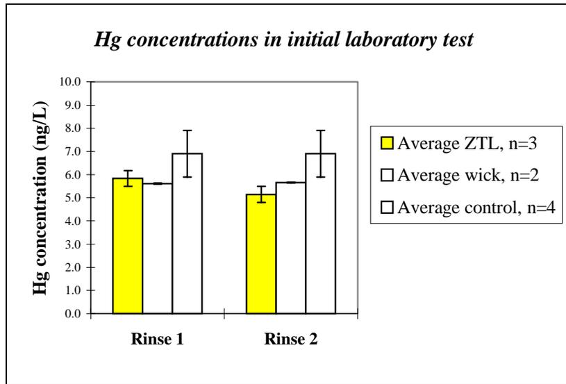
**Figure 1.** Results from the first laboratory test comparing Hg concentrations in rain water (control) vs. water poured through ZTL and wick devices. Error bars represent one standard error of the mean (not visible for wick because of small sample size and consistent results).
