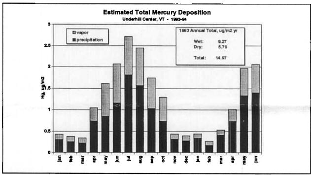
Figure 2. Wet and dry deposition of Hg from precipitation and estimated vapor deposition at Underhill Center, Vermont, in 1993 and 1994.
