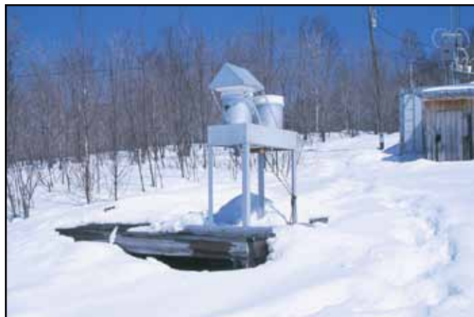
Aerochem precipitation collector used to collect AIRMoN precipitation samples at the Proctor Maple Research Center’s Air Quality site.
