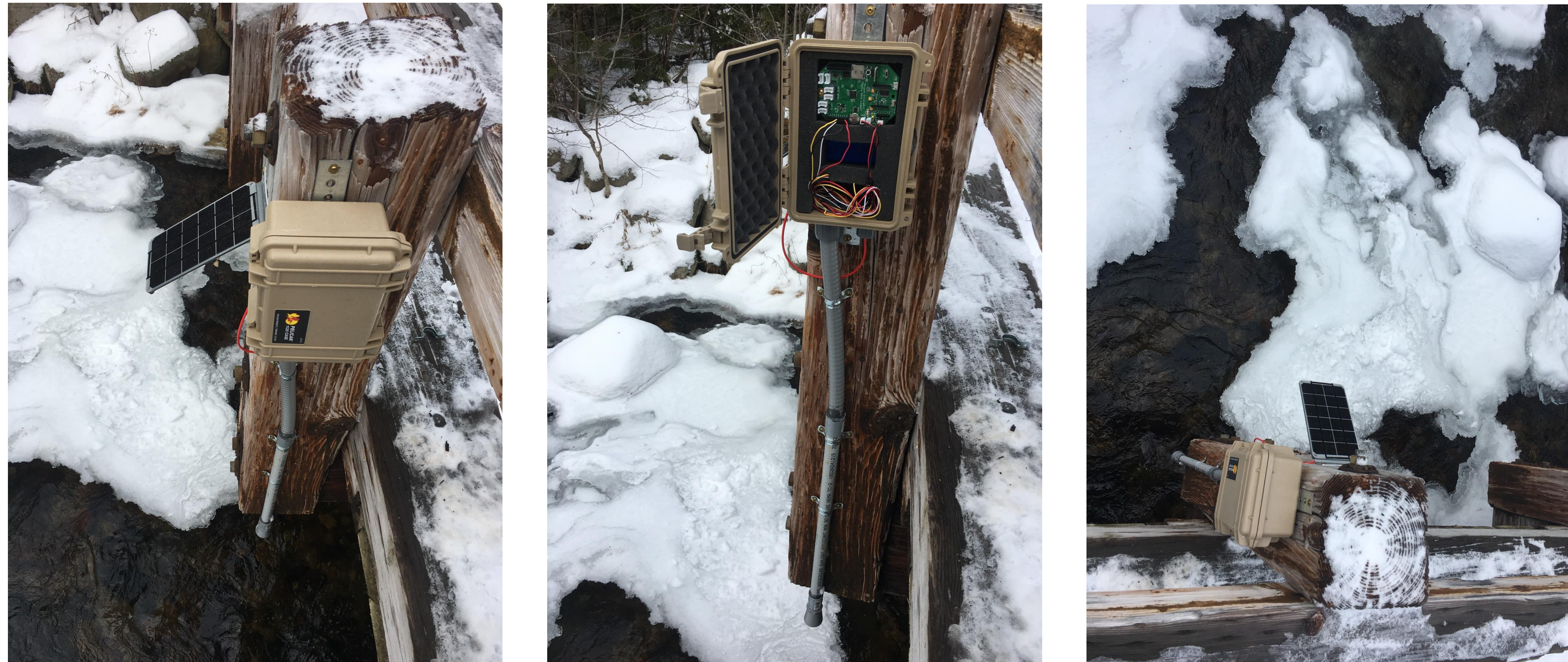
Stream gaging station installed on bridge at Wildcat Brook, Jackson, NH
