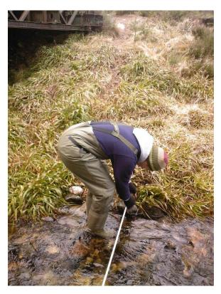
Figure 16. Measuring Stream flow.
