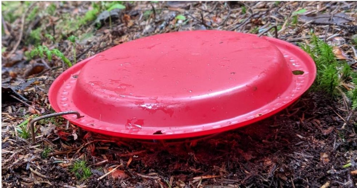
Figure 3: Plastic plate cover suspended ~1" off the ground by two landscaping staples (one of which is visible) to protect the underlying pitfall trap from filling up with rainwater and leaves. The ¼" holes along the edge of the plate are for rain drainage. ©Jason Hill.
