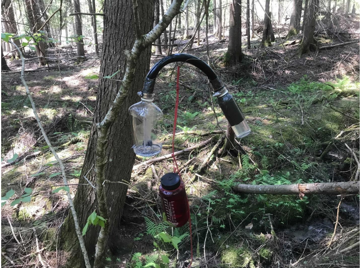
Figure 2. Our initial attempt at developing a cost-effective modified window trap in 2021 for sampling aerial insects. Our design was prone to blowing about in the wind, and we attached weights (e.g., a filled water bottle) to increase the stability of our trap in the wind. ©Pete Kerby-Miller.
