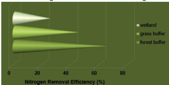
Figure 2. Nitrogen removal efficiency (%) between wetlands, grass buffers, and forest buffers.
