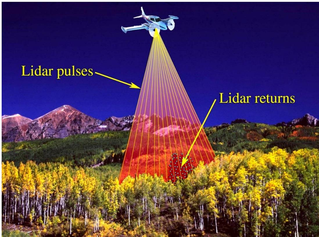
*Figure 28. Graphic showing how lidar pulses reflect off of objects and return to the receiver. From presentation by Jarlath O'Neil-Dunne.*
