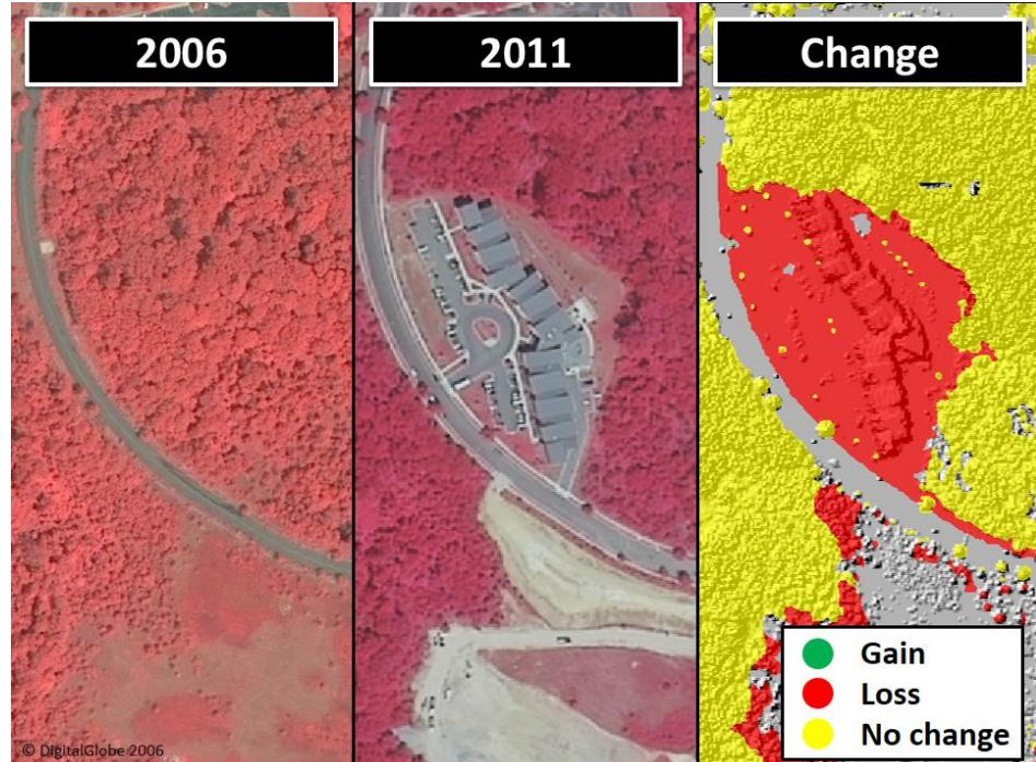
Figure 16. Mapping land cover change using LiDAR and emerging remote sensing analytical tools. From presentation by Sean MacFaden.
