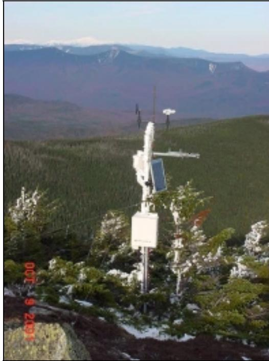
**Figure 3.2.** High elevation site (1425 m) on Mt. Moosilauke, early October 2001. Accumulated rime ice can be seen on the support pole and anemometer cup. Mt. Washington is the large, snow-capped peak seen in the far distance.
