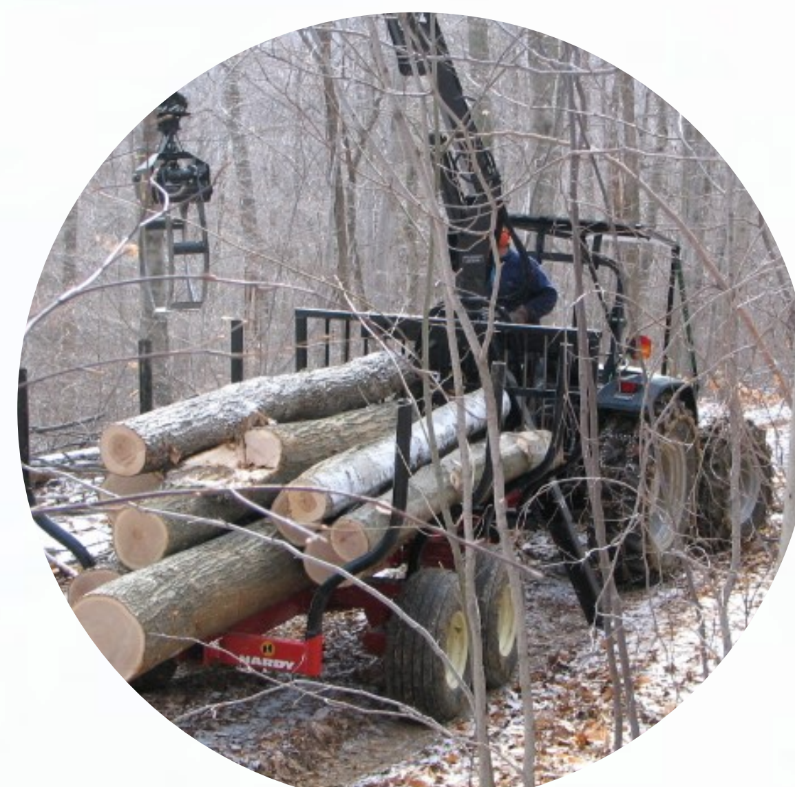
Bill Torrey uses a forwarder to collect logs in the forest. Forwarders are much lighter on access paths than skidders, which drag logs.
