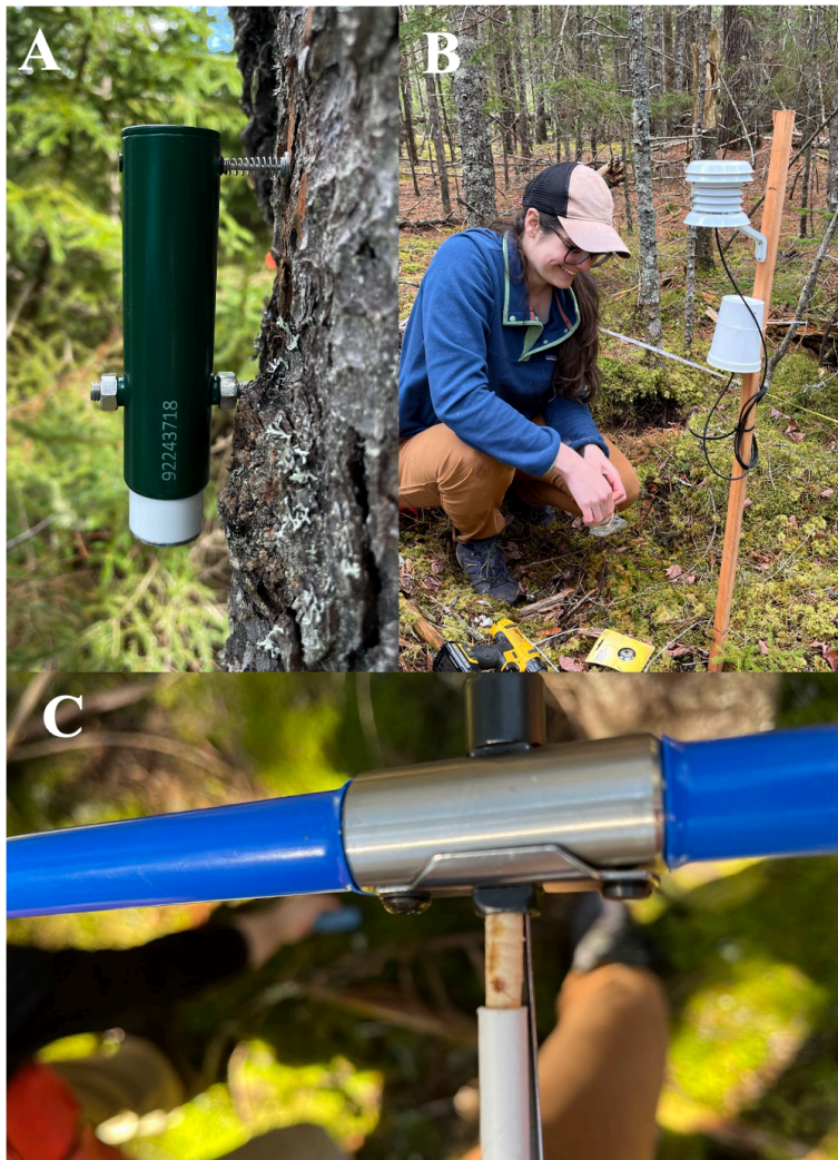
Figure 2: A: Photo of an automated point dendrometer deployed on a red spruce tree. B: Photo of a HOBO climate sensor mounted to a wooden stake. C: Photo of increment core being extracted from a red spruce tree.
