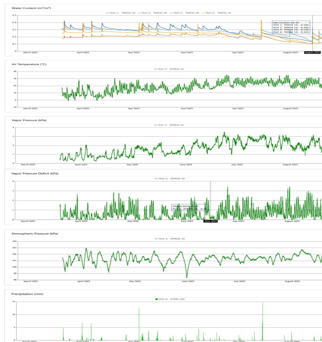
Figure 6: Weather station data representing (top to bottom), soil moisture at two depths in two locations, air temperature, vapor pressure, vapor pressure deficit, atmospheric pressure and precipitation in 15-minute intervals from March 19 th to August 20 th 2025.
