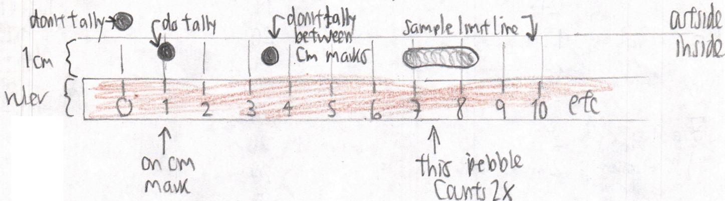
Use 100 cm = 1m to convert directly into % without any calculations. If stones are maximally in part of the sampling criteria (i.e. directly on the edge), tally every OTHER stone. Cm are better than inches because a smaller exposure is required, 39.37" = 1m rather than 100 inches => 8 feet.
