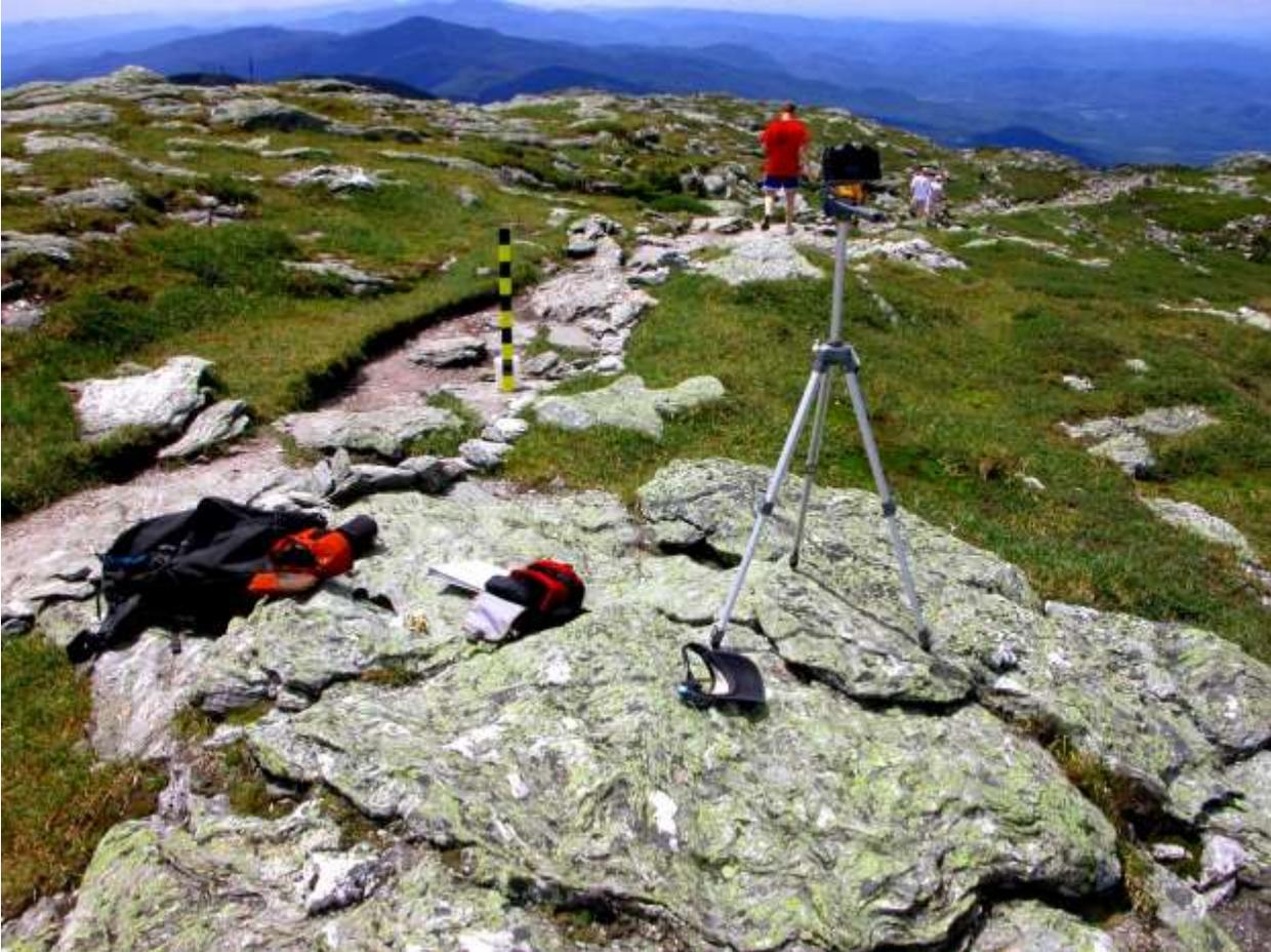
Standard phototranssect setup: Camera and tripod on right, meter board 5 meters away on left.
