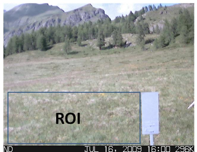
**Fig. 2.** Digital image collected by the CC640 Campbell camera the 16th July 2009. Blue box denotes the static Region of Interest (ROI) selected for the study. The grey reference panel is visible on the bottom right portion of the image.
