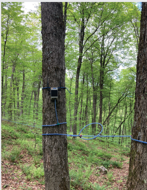
Monitors throughout the sugarbush identify the location of vacuum leaks
