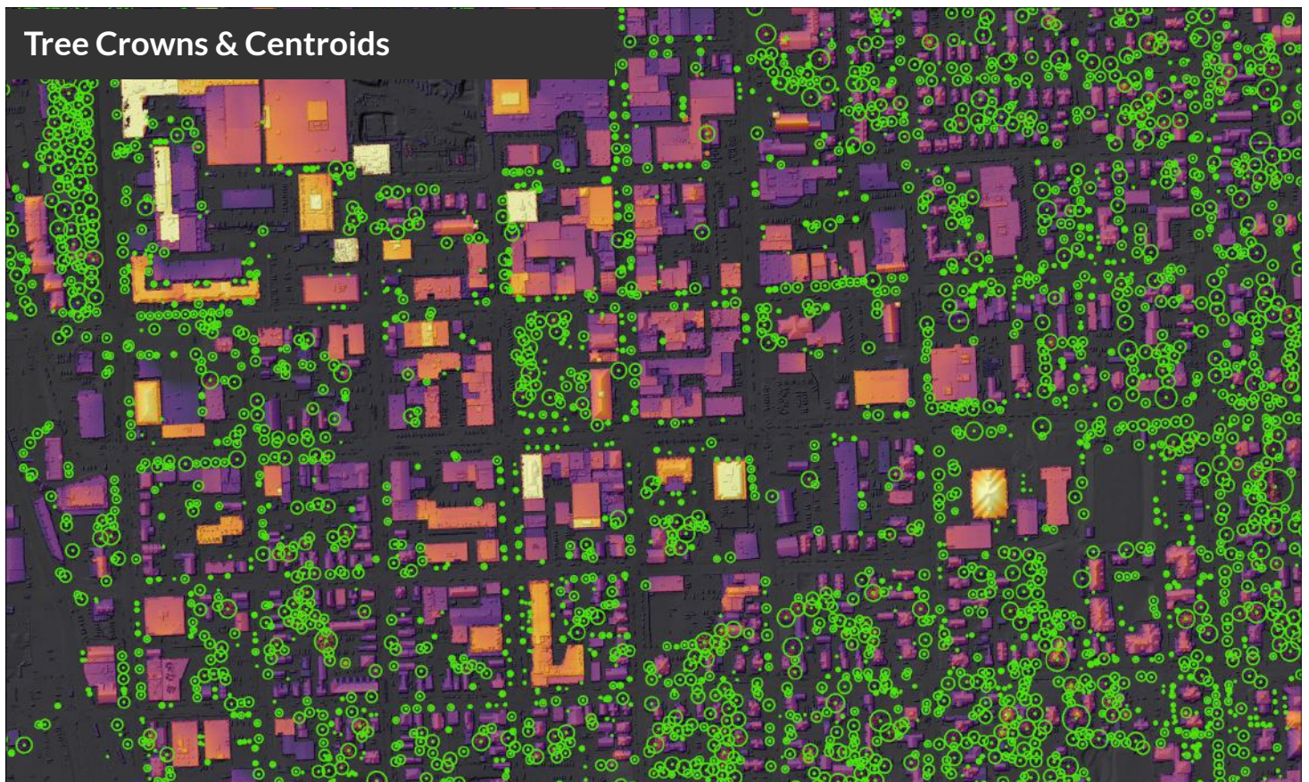
Figure 3. Tree centroids (dots) and tree crowns (circles) mapped from the 2023 LiDAR. Tree mapping from LiDAR involves finding relative high points for each tree, then tracing down until a height inflection point is reached, marking the edge of the crown. This approach to individual tree mapping is most accurate where there is a clear differentiation in tree crowns and is less accurate in forested stands where crowns may overlap.
