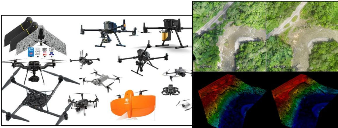
*SAL UAS fleet and data examples (true-color mapping and LiDAR elevation) from a 2024 landslide*
