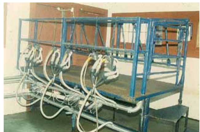
Photo 9.6 Prefabricated elevated parlor.
