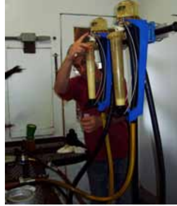
Photo 5.1 (LEFT) Technician setting up milk meters in parlor so meters are level.
