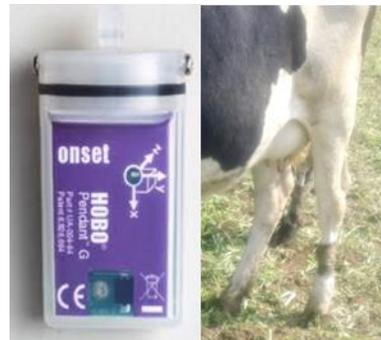
A number of research studies have been conducted using Hobo Pendant® accelerometer data loggers (Onset Computer Corporation, Bourne, MA) to monitor cow behavior. These data loggers collect positional information which can be converted to assess walking and lying behavior. Most past research using this tool has focused on cattle in confinement housing.
