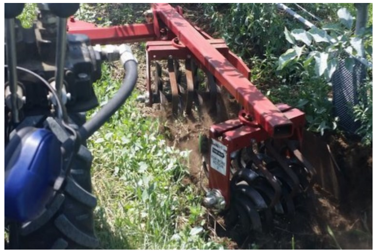
Figure 6. Wonder Weeder™ ground-driven under-tree cultivator, Harris Mfg., Burbank, WA.
