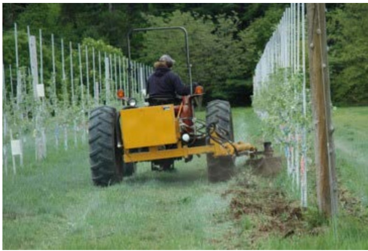
Figure 5. Hydraulic rotary cultivator (Weed Badger™, Marion, ND).
