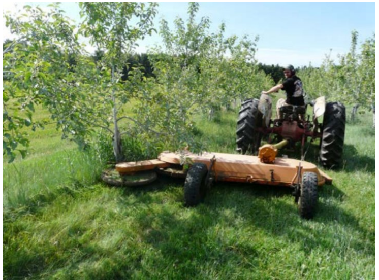
Figure 2. Mowing semidwarf trees with a swing-arm mower.
