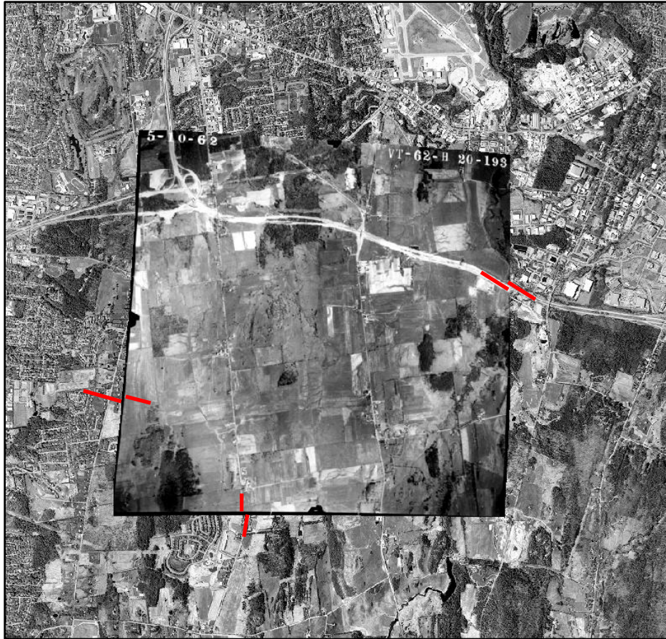
Figure 5. This image shows a rectified 1962 aerial photo atop a 2011 aerial photo. The 1962 image has been stretched to the dimensions of the 2011. The red lines on the photos show where roads should match but do not. GCPs need to be added in those areas to achieve a more accurate rectification.
