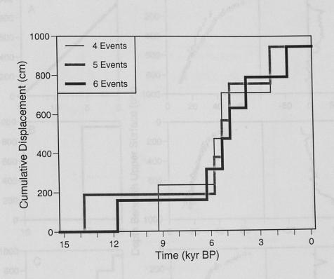
Figure 11. Cumulative displacement versus time for best fit histories of 4, 5, and 6 events. All three of these histories show most displacement occurs for a relatively short period of time, centered around 5 kyr BP. Lesser amounts of displacement occur between 14 to 11 and 1 to 2 kyr BP.
