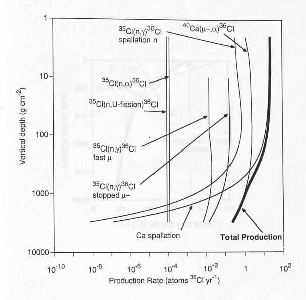
Figure 7. <sup>36</sup>Cl production rates at depth for the seven production pathways, assuming 10 ppm Cl in pure calcite (CaCO<sub>3</sub>). <sup>40</sup>Ca spallation is the dominant production pathway in the upper 3 m, <sup>40</sup>Ca muon capture dominates below 3 m (Section 4). Actual production rates for individual samples vary according to chemical composition. Figure after Stone et al., 1998.
