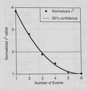
Figure 13. Lowest residual  $(x^2)$  value for each displacement history series. For comparison,  $x^2$  values have been normalized to the lowest residual. Higher numbers of events results in better  $x^2$  values; however, the change in  $x^2$  decreases with an increasing number of events.
