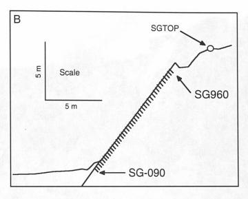
Figure 4. A. Scarp cross section at sampling location. Vertical offset is calculated by measuring the vertical distance between the top and bottom of the scarp (Figure 2). Section A to A' is shown on Figure 3. B. Close up diagram of the Nahef East fault scarp, showing a small slab of chalk covering the base of the scarp. Scarp sample locations are marked by tick-marks, and sample SGTOP is marked with an open circle.
