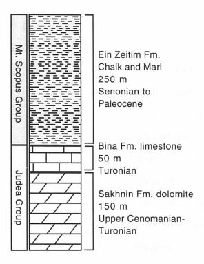
Figure 2-1. Simplified stratigraphic column of the Galilee, including rock units found adjacent to the Nahef East fault. The Senonian chalk has been dropped at least 50 meters and is now found next to Turonian carbonates.
