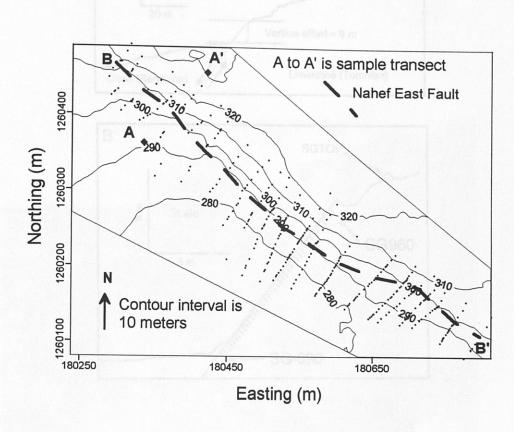
Figure 3. Topography of the Nahef East fault scarp and the surrounding area (Israel Map Grid, contours in meters asl). Constructed from GPS data points. A to A' are the ends of the scarp cross section sampled for <sup>36</sup>Cl (Figure 4), B to B' are marked on the displacement vs. distance diagram (Figure 2). Small dots are transects used to measure scarp displacement (Figure 2).
