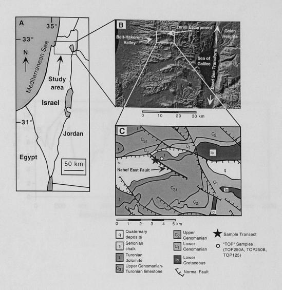
Figure 1. A) Location, B) topography and C) geology of the Nahef East fault scarp. Location of "TOP" sample shown by the open circle in C. Digital shaded relief image from J. Hall, Israel Geologic Survey Shaded Image Relief Map, 1:500,000, 1991; geologic map after Geologic Survey of Israel Geological Map, 1: 250,000, 1965.
