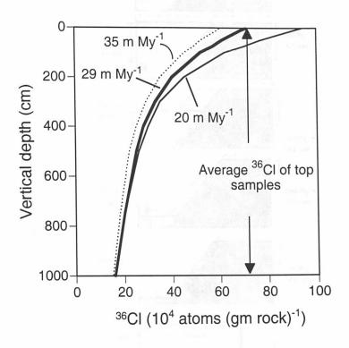
Figure 8. <sup>36</sup>Cl in the upper samples as they are exhumed at different erosion rates. An erosion rate of 29 m My<sup>-1</sup> results in a <sup>36</sup>Cl concentration of 71 x 10<sup>4</sup> atoms (gm rock)<sup>-1</sup>, the measured value. Samples were taken from an elevation of 300 m, and a latitude of 33°. All seven production pathways (Figure 7) were used to calculate the erosion rate.
