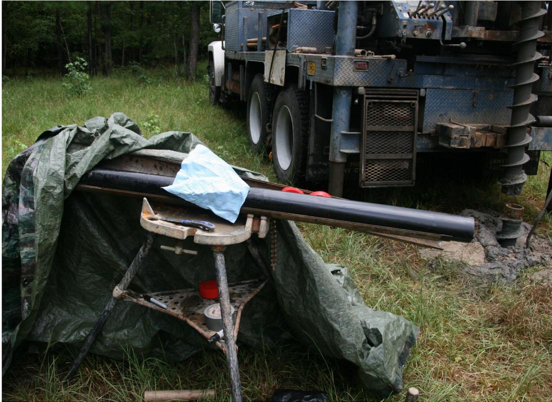
Figure 2-7 (SD2) OSL field sampling setup. Painted core liner is shown inside split inner core barrel. Sediment cores were collected and packaged under the tarp for transport to the laboratory without being exposed to light.
