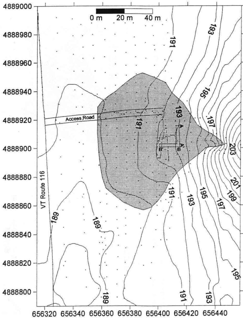
Figure DR2B. Topographic map of Bristol fan. X and Y axes are in UTM coordinates. Contour interval is 1 meter. Dots are measured survey points. A-A' and B-B' are trench locations.
