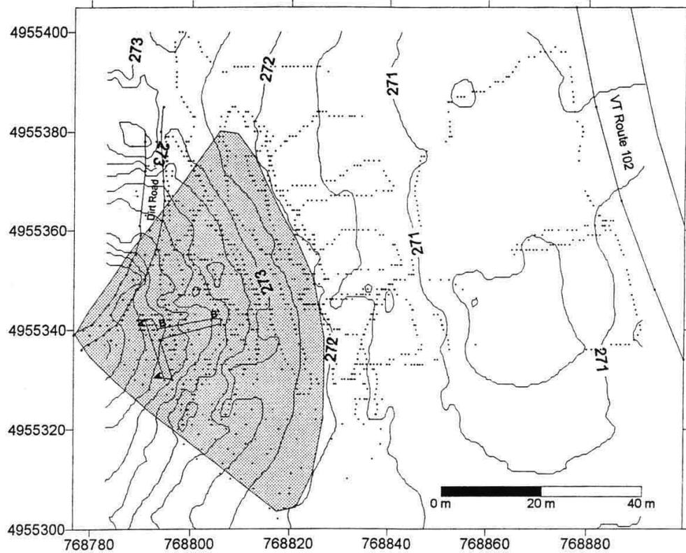
Figure DR5B. Topographic map of Maidstone fan. X and Y axes are in UTM coordinates. Contour interval is 1 meter. Dots are measured survey points. A-A' and B-B' are trench locations.
