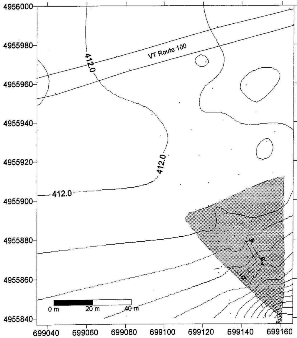
Figure DR1B. Topographic map of Eden Mills fan. X and Y axes are in UTM coordinates. Contour interval is 0.5 meter. Dots are measured survey points. A-A' and B-B' are trench locations. Dashed line is stream channel.
