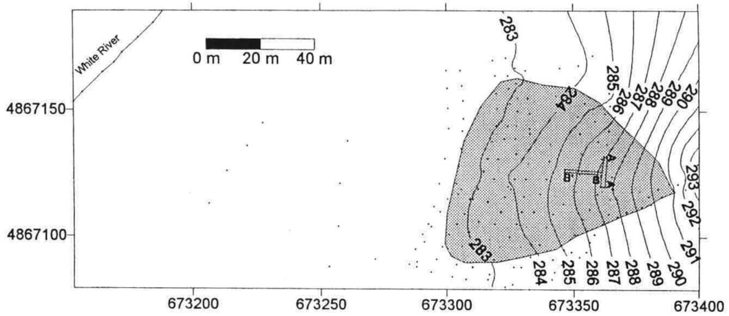
Figure DR3B. Topographic map of Hancock fan. X and Y axes are in UTM coordinates. Contour interval is 1meter. Dots are measured survey points. A-A' and B-B' are trench locations.
